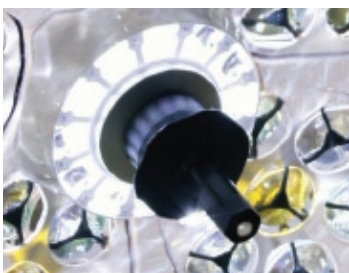
State-of-the-Art HYBRID (Fixed and Focusable) LED Optics
